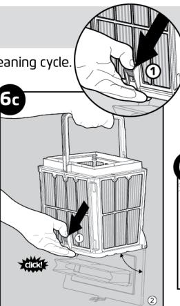
Open the latch to release the bottom lid in order to remove the debris.
